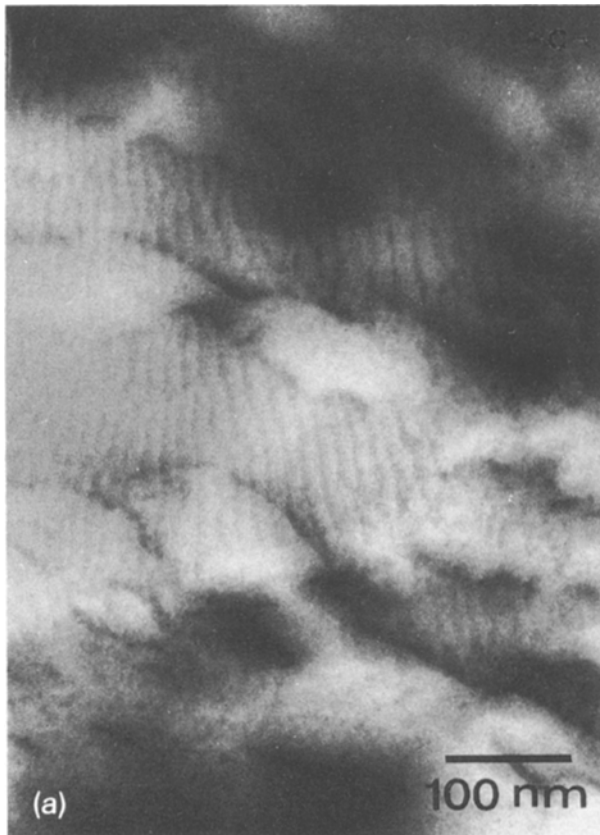
Figure 5 Structural defects in ceramics sintered at 1373 K for 1 h (a) and 16 h (b).
